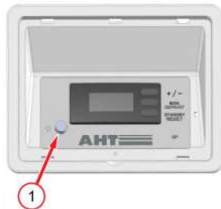
Fig. 4: Appliance lighting switch (1)
